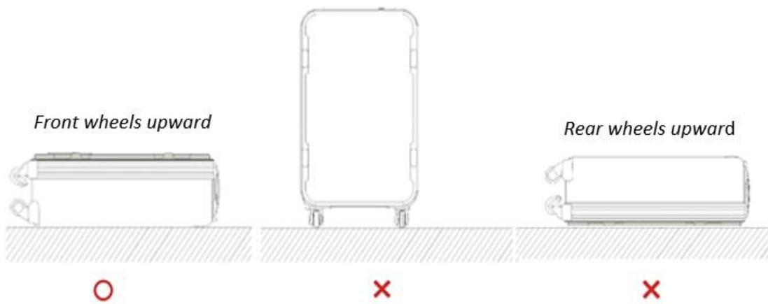
**Figure 7. Physical Positioning for Transportation in a Vehicle**
