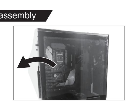
**English** Remove the screws on the back of the chassis, and open the side panel.
